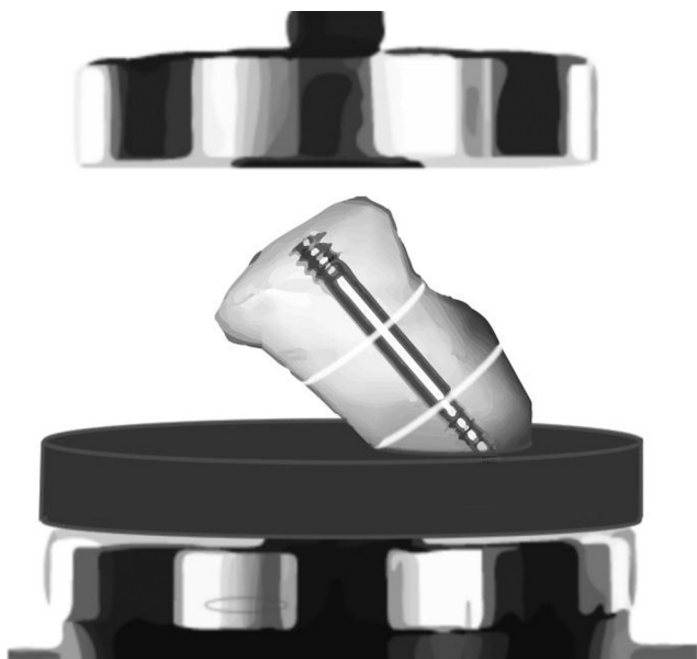
Fig. 2. A cadaveric scaphoid nonunion model fixed with headless compression screws was tested with an Instron ® tensile testing machine.
