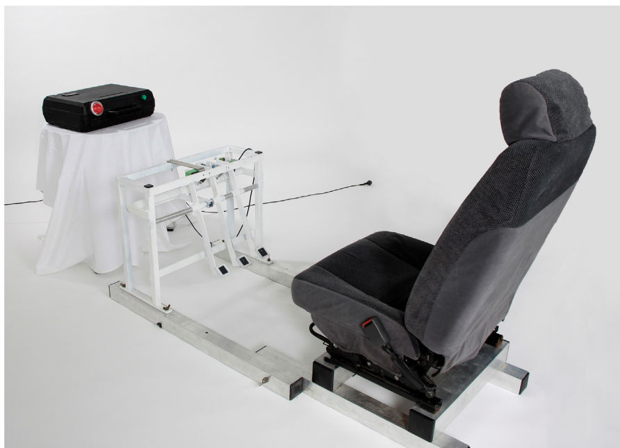
Fig. 1. Custom-made apparatus for measurement of brake reaction time (BRT). Pedals from left to right: coupler pedal; brake pedal; accelerator pedal. External suitcase: red light: (visual stimulus initiating the braking procedure); green light: (indicating that the accelerator is fully depressed – subject not in a 'ready-to-brake fashion'). (For interpretation of the references to colour in this figure legend, the reader is referred to the web version of the article.)
