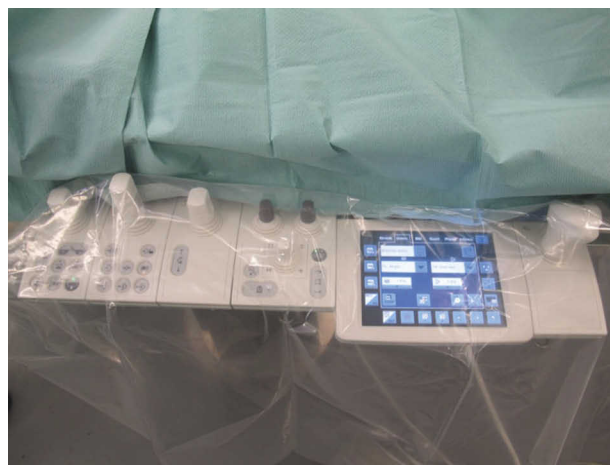
Fig. 2. Control panel of the c-arm. The system is able to be completely controlled by the surgeon.
