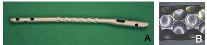
Fig. 1. Intramedullary nail in total view (A) and in detail showing the “golf ball” structure of the surface (B).
