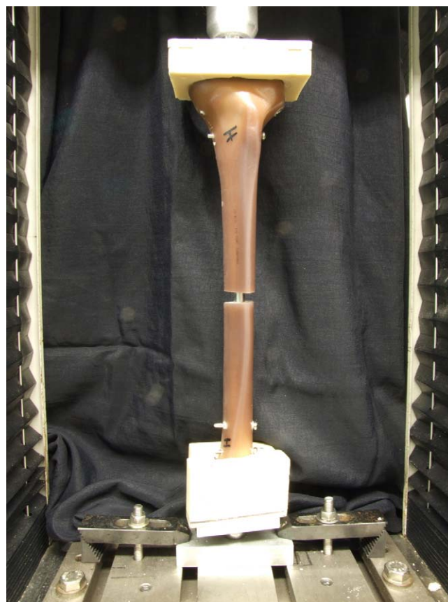
Fig. 2. For axial and cyclical axial testing, the proximal and distal end of each tibia was held in a PMMA mould and supported by a ball bearing in the materials testing machine to avoid uncontrolled torque or bending.
