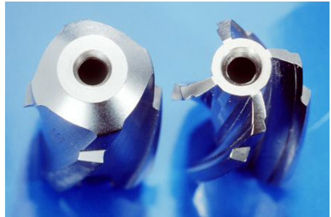
Fig. 1. Reaming systems with different reamer heads. The experimental reaming system contains a reamer head with deepened cutting flutes and a reduced drive shaft.
