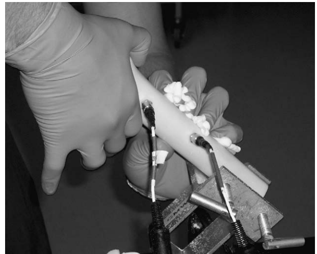
Fig. 2. Visualised cement escape in a pre-drilled femur, the two drilled sensors are seen.
