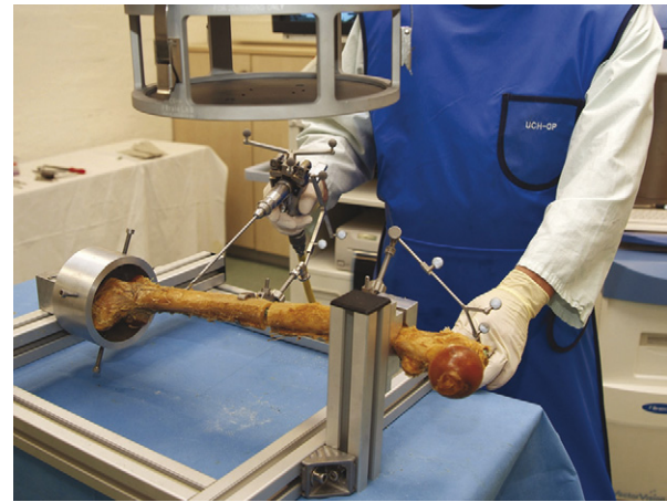
Figure 1 The custom femur holding apparatus allowed for immobilisation of the proximal segment and nail, while the distal fragment was free to rotate.
