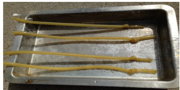
Figure 2. 13 × 9-inch baking pan with the tied tubing taped to the base and the open end taped to the upper rim.
