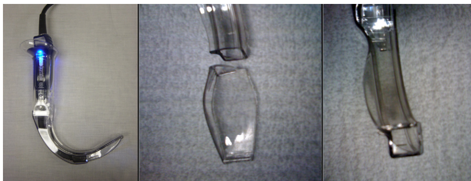
Figure 1. New GlideScope® Cobalt with GVL® Stat (left), fractured GVL® Stat (middle and right).
