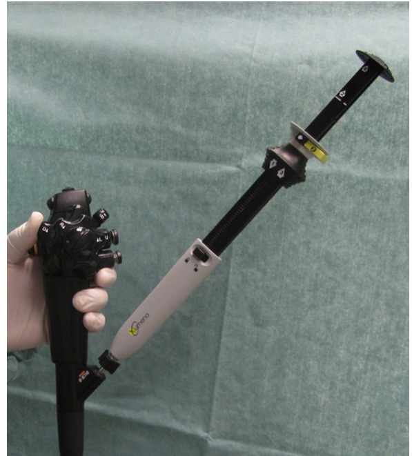
Fig. 2. The handle of the AXIOS delivery system is Luer-locked onto the echoendoscope instrumentation channel inlet port, analogous to a standard fine needle aspiration needle. The handle consists of a distal portion for catheter control and a proximal portion for stent control.
