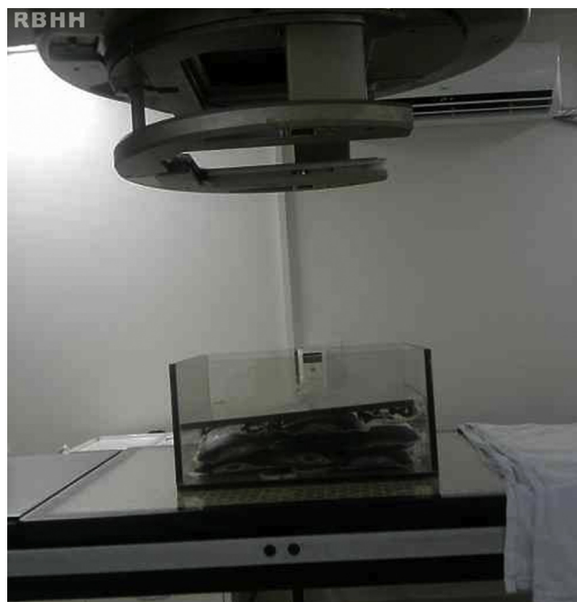
Figure 1 – Polycarbonate container designed to irradiate packed red blood cell bags.
