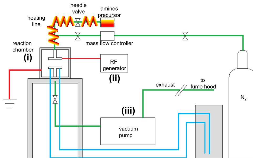
Fig. 1. Plasma polymerization apparatus which is composed of (i) reaction chamber, (ii) RF generator, and (iii) pumping system.
