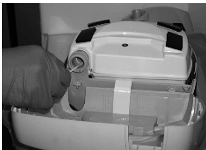
Figure 1. Swabbing the non-invasive ventilation device air outlet: outer area.
