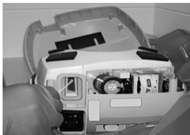
Figure 2. Swabbing the non-invasive ventilation device air inlet filter housing.
