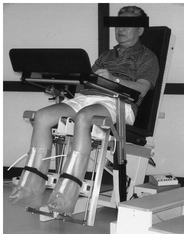
Fig. 1. Experimental setup for the assessment of knee joint proprioception, showing the measurement chair control mechanism, handheld button, air splints, and footrest (the moving component of the apparatus).
