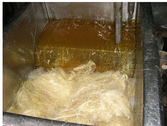
Fig. 2. 200-L pilot plant tank where the cut flax fibers were placed next to the housed-propeller that moved the fibers up and down.
