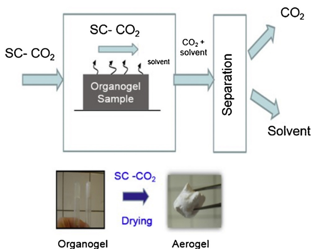
Fig. 1. Simplified scheme of supercritical drying.
