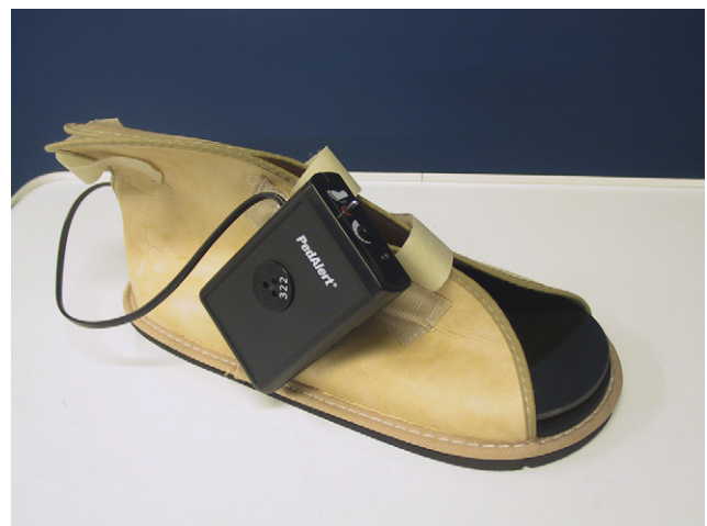
Fig 1. The Pedalert audio feedback system.
