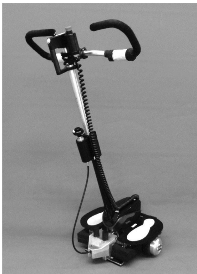
Fig 1 The PTAR is a stand-up-and-ride transport robot and a personal mobility device with 2-wheel inverted balancing, which moves by transferring the rider's COG.
