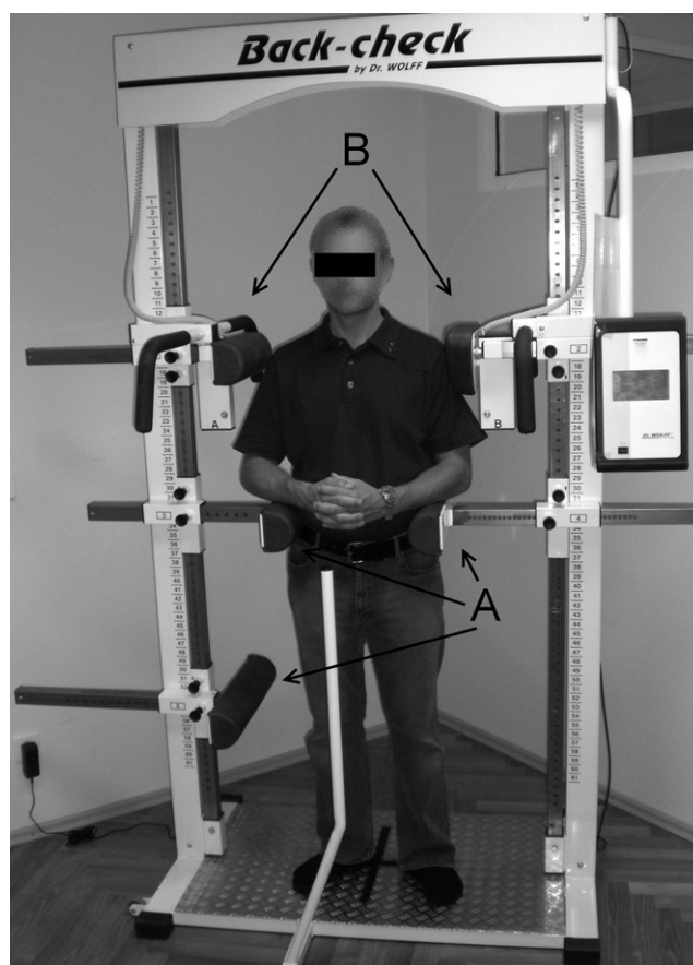
Fig 1. Back Check 607—lumbar lateral flexion left. (A) Three adjustable arms for fastening the subject. (B) Two adjustable measuring mechanisms.
