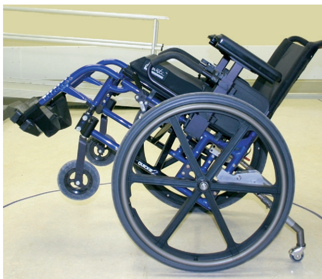
Fig 1. The Arc-RAD–equipped wheelchair, tilted back and resting on the Arc-RADs. The casters are off the ground.
