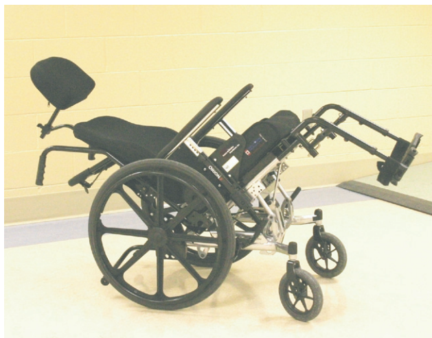
Fig 2. The tilt-in-space wheelchair, tilted back. The casters are on the ground and the conventional rear anti-tip devices are off the ground.
