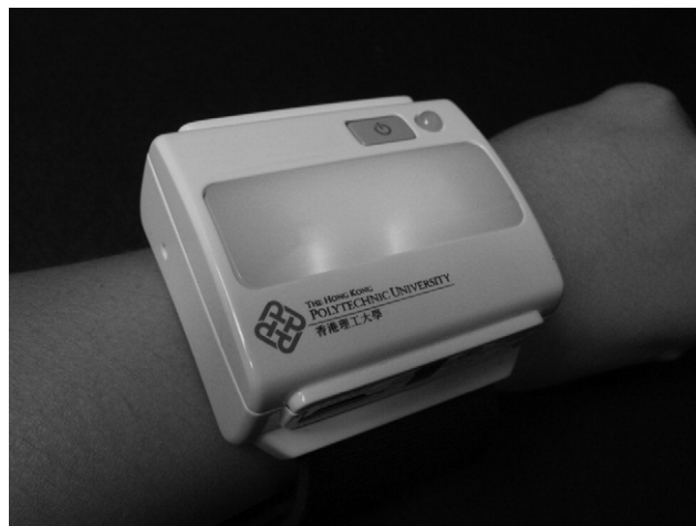
Fig 1. View of the device from above to show the acknowledgement button and how it is worn on the wrist.
