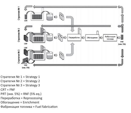
Fig. 1. Flowchart for the VVER-1000 reactor conversion to reprocessed uranium for the three strategies.
