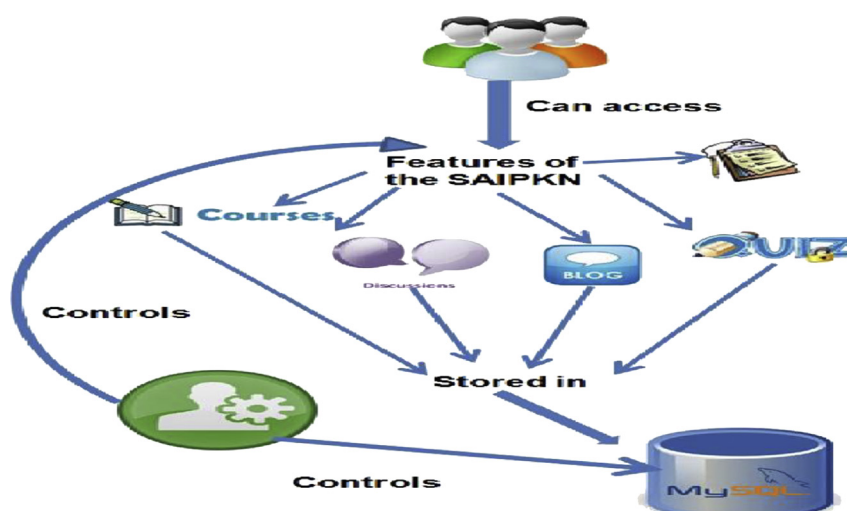
Fig. 2. How SAIPKN works.
