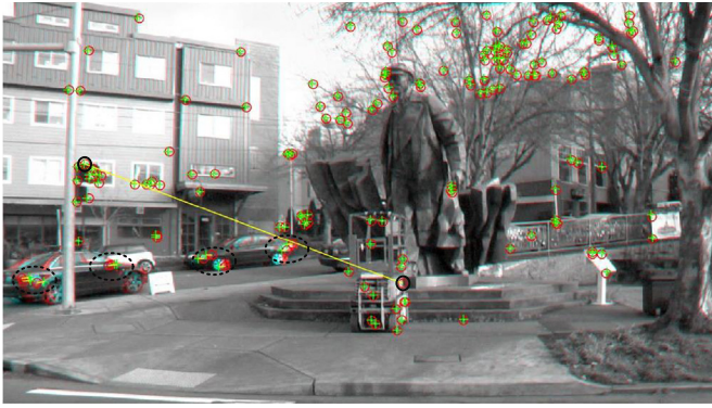
Fig. 1. FREAK descriptors from frame 361 and frame 362 in video sequence “Statue”. The lines across the symbol \circ and symbol + represent the connections of matched features. The solid and dotted black circles represent the incorrect-matched and inconsistent feature points, respectively.
