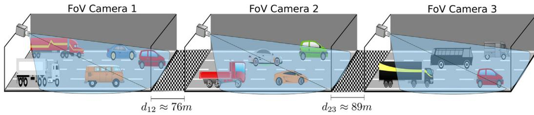
**Fig. 1.** Example of a multicamera setup for tunnel surveillance with non-overlapping views. Vehicle re-identification is needed to correctly associate each of the vehicles across different cameras installed in the tunnel.
