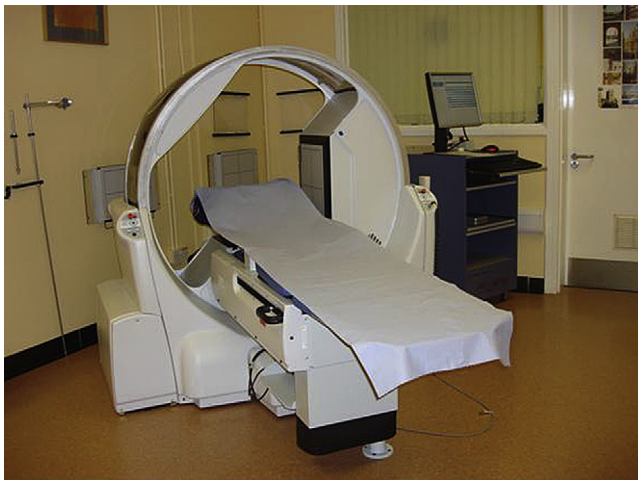
Figure 1 Typical modern sodium iodide gamma camera designed for dedicated cardiac work. The sodium iodide crystal heads are perpendicular to each other and rotate around the patient’s heart in 32 steps. Collimators in front of the heads allow only perpendicular photons through to the crystals. The resulting scintillation is amplified by photomultiplier tubes and converted to an electrical signal that is gated to the patient’s ECG. Transaxial slices are created, reconstructed to standard orthogonal planes and displayed on the computer workstation. Fixed planar imaging (non-rotating camera heads) is no longer used for MPS work; SPECT (single photon emission CT) is preferred especially as this allows functional assessment.
