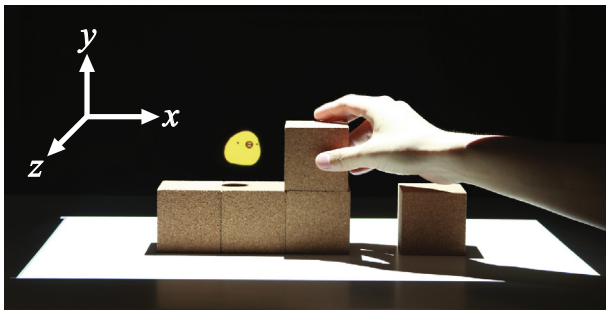
Fig. 1. The MARIO system. Users can directly interact with physical objects and mid-air images. A virtual character (Hiyoko, a chick) is displayed in mid-air over wooden blocks. A coordinate system is defined as x for width, y for height, and z for depth.
