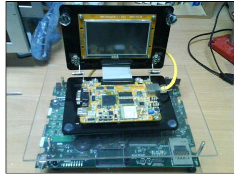
Fig. 2. Distributed dual-platform DaVinci+NAV270.
