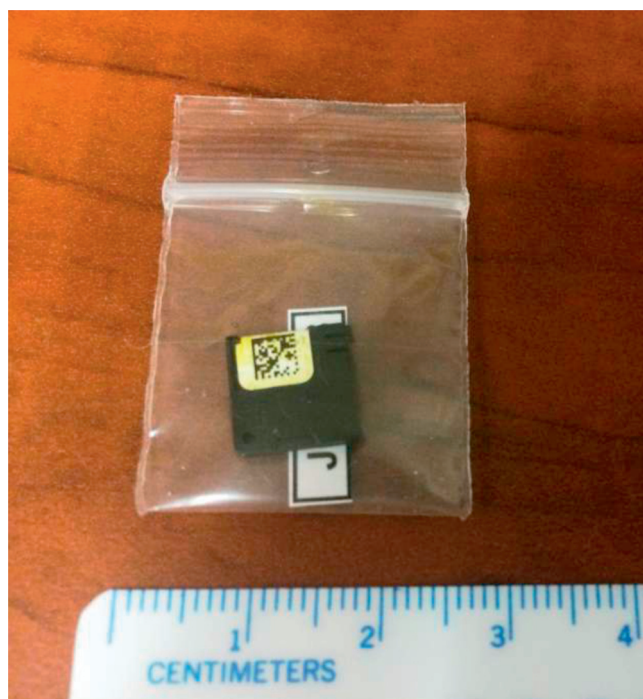
Figure 1. nanoDot thermal leak detector (ie dosimeter for measurement of skin entrance radiation doses).
