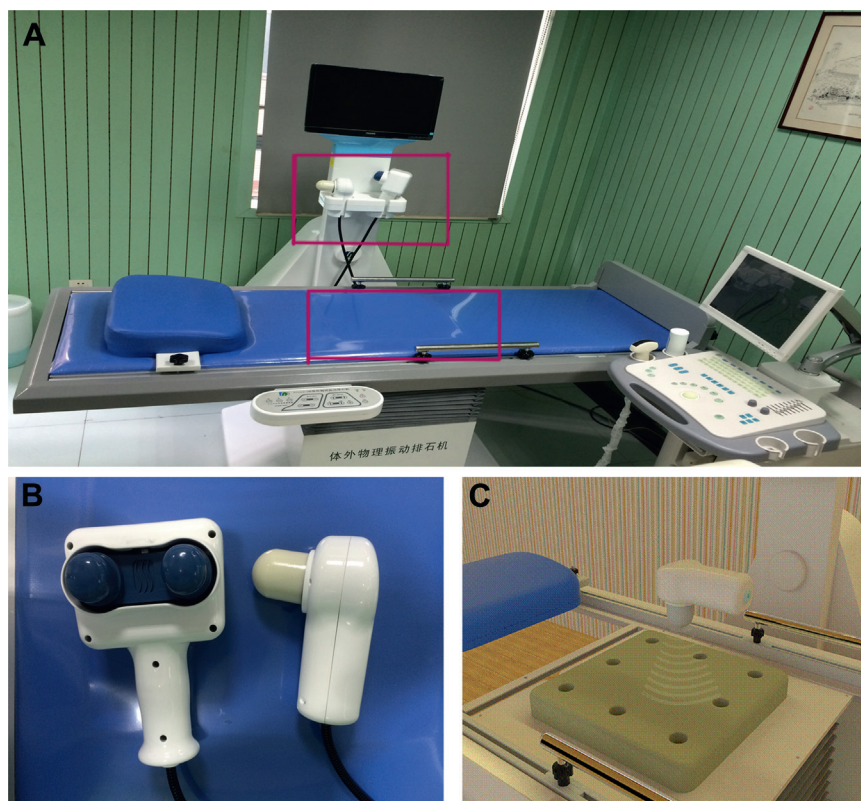
Figure 1. Prototype of Friend-I EPVL, showing whole view (A), master oscillator (B) and associate oscillator (C)
