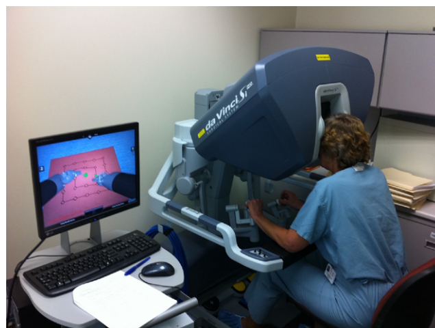
Figure 1. da Vinci Skills Simulator prototype integrated with da Vinci Si Surgeon Console.
