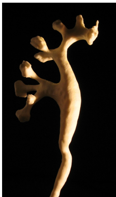
Figure 1. Right renal collecting system model created by rapid prototyping.
