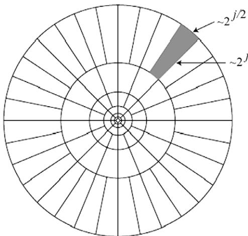
Fig. 1. Continuous curvelet support in the frequency domain.
