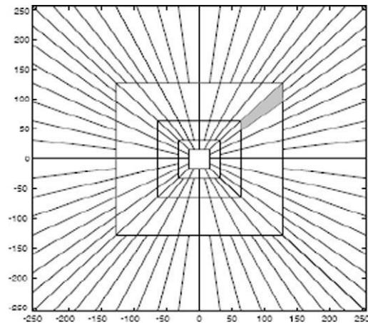
Fig. 2. Digital curvelet tiling of space and frequency.
