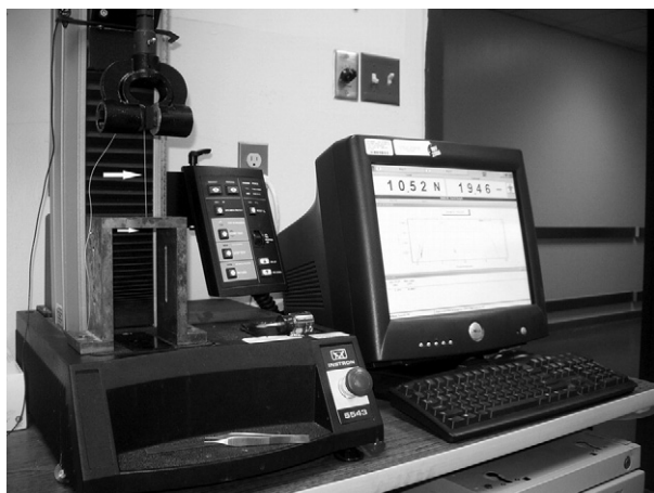
Figure 1. The Lapra-Ty clip (small arrow) was applied to the distal 1 cm of suture. The proximal end of suture (large arrow) was passed through a 2-mm hole in the metal stand and secured to the AMTS arm.
