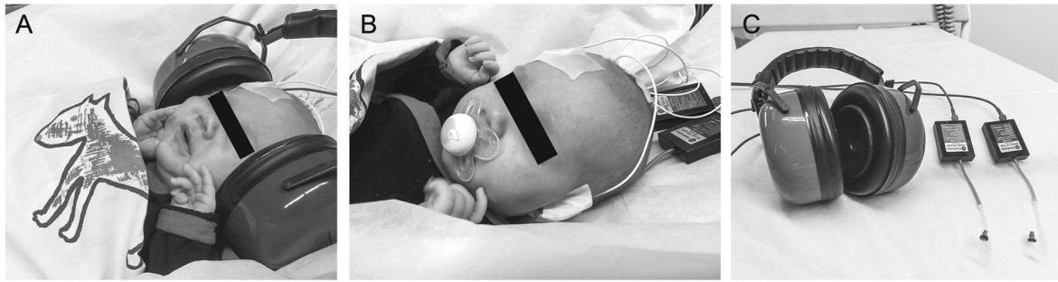
Fig. 1. Set-up for neonatal BAEP and BA recording performed with traditional headphones (A) and tubal insert earphones (B). Headphones and TIPs at a closer view (C). The length of the silicon tube in TIPs is 153 mm and in our department the length is monitored regularly.
