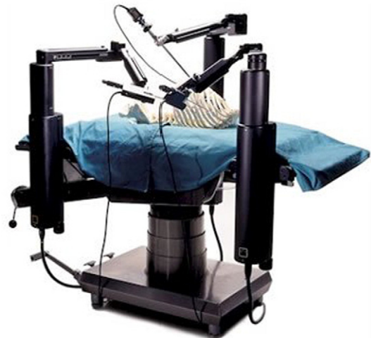
Fig. 3. ZEUS robotic system; first robotic system to combine instrument and camera control.
