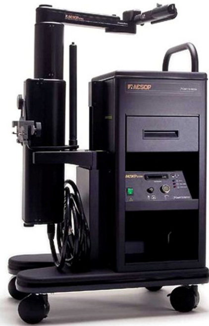
Fig. 2. Computer Motion's AESOP (Automatic Endoscopic System for Optimal Positioning) has allowed surgeons to control the orientation of the laparoscope via foot pedal and later voice commands, freeing both hands for surgery.
