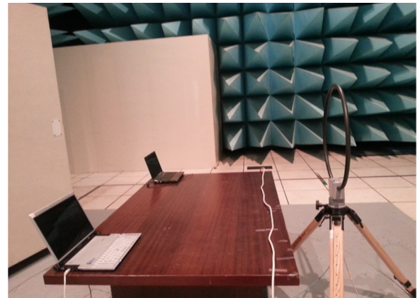
Fig. 3. Configuration for radiated emission.
