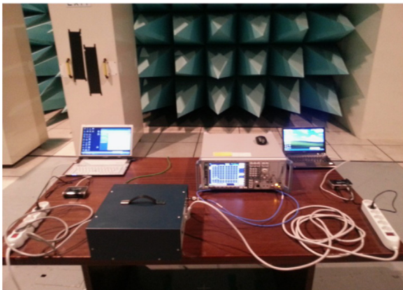
Fig. 1. Configuration for conducted emission.
