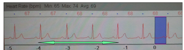
Figure 2 Example ECG to show predicted HRV as calculated by the scanner (67 + 68 + 68) / 3 (green arrow). Image acquisition corresponds to the blue box. The beat prior to the acquisition is not assessed as table feed has commenced.
