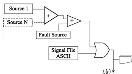
Fig. 1. Signal generation module.
