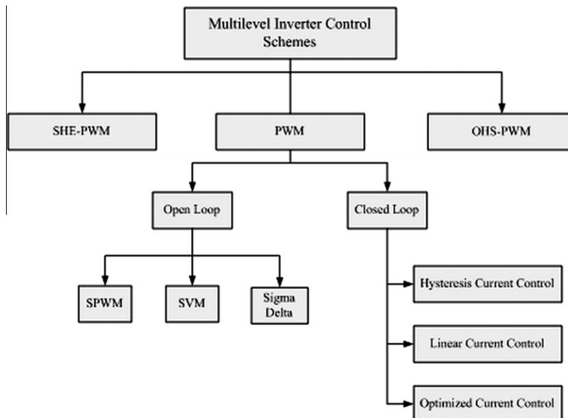
Fig. 1. Classification of multilevel inverter control schemes.
