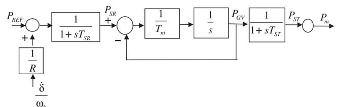
Fig. 2. IEEE steam turbine speed governing system.
