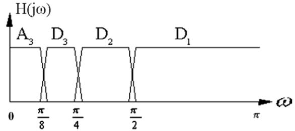
Fig. 3. Three-level DWT frequency band.
