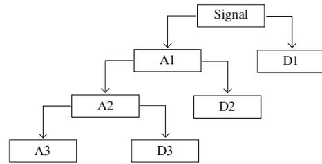
Fig. 2. Three level decomposition signal in DWT.
