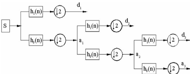
Fig. 1. DWT multiresolution algorithm.
