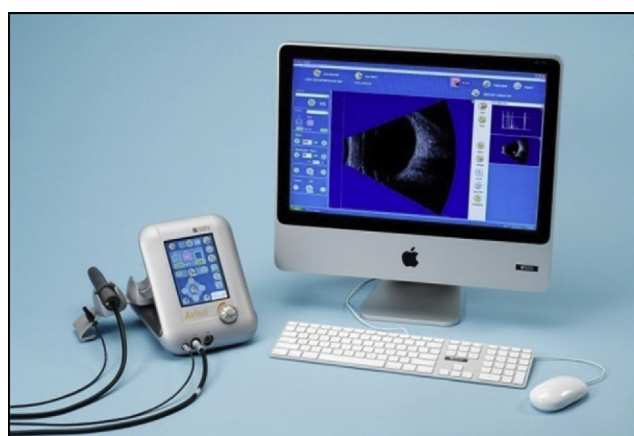
Fig. 1 – Ophthalmic echography equipment: Aviso de Quantel Medical®, comprising a 10 MHz probe for ultrasound mode B and probe for standardized mode A.
