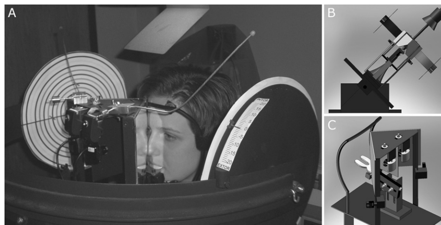
FIG 1. Haploscope. The device fully illustrated in 3 views. (A) Photograph with subject viewing. Note the angled mirror configuration, overhead lamp, bite bar, left and right cameras, and opposed viewing targets. These near targets at a 33 cm viewing distance each provide a field of view greater than 50°. (B) Illustrated front view, tilted right. Note the overall device design with wide base, capable of tilting 45° to the subject's left and right. (C) Illustrated oblique view, close-up. Note the configuration of the infrared cameras, which are mounted facing the subject, behind the angled mirrors.
