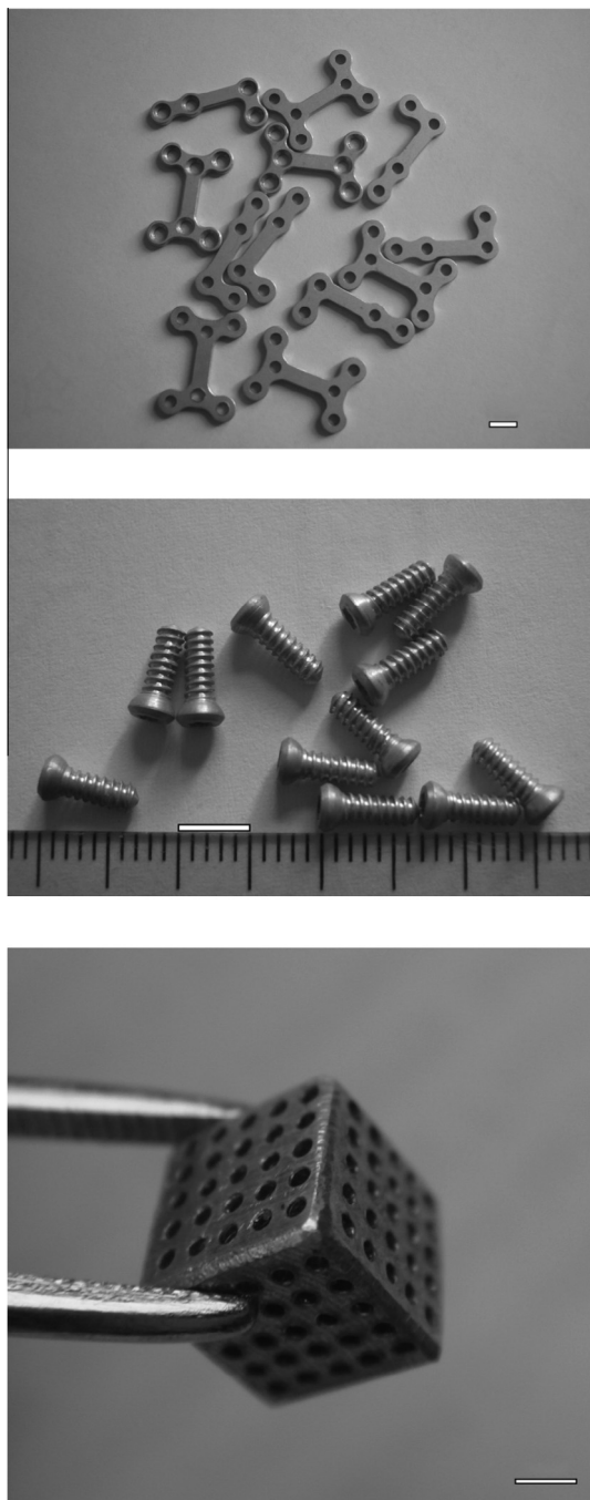
Fig. 1. Biodegradable orthopedic devices prepared from Mg and its alloys: (top) bone plates; (middle) screws for orthopedic fixation; (bottom) a porous scaffold for bone void filling. Scale bar = 10 mm. Reprinted from Ref. [14] with permission.
