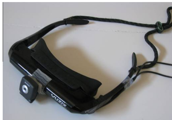
Fig. 1. An image of the pixelized vision simulator which consists of a USB camera and miniature LCD monitors mounted on goggles.
