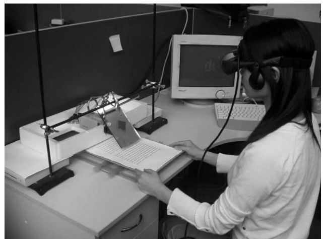
Fig. 1. Setup of the pixelized reading task. Through the reflection mirror, the video camera captured images of the reading materials placed on a moveable paper tray. The captured images were degraded into low resolution and transformed into simulated phosphenes patterns in real time. A head-mounted display presented pixelized images to the subject. This picture shows a subject reading with manual page navigation with this simulation system.
