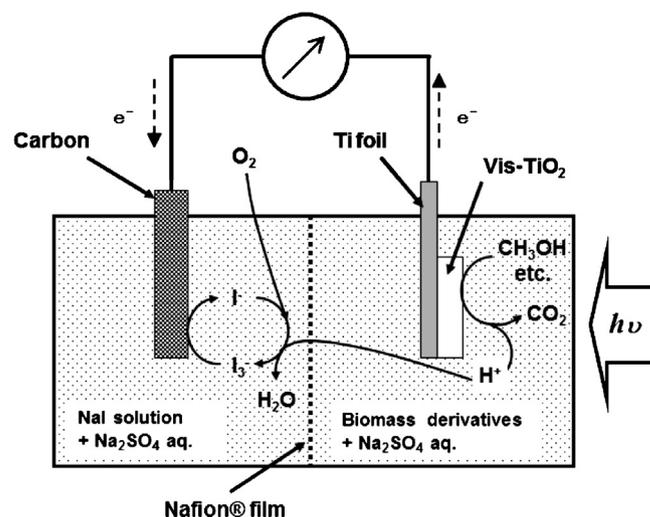
Fig. 1. A scheme of electric power generation by using a separate type photofuel cell (SPFC).
