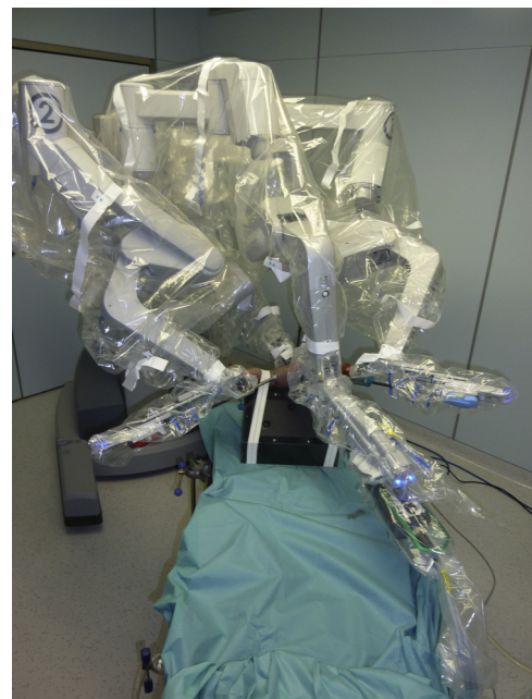
Fig. 2. Installation of the telemanipulator. The arms of the Da Vinci ® robot were linked to the trocars in which the instruments and the camera were introduced.
